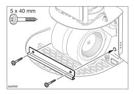
Secure the canopy by guiding the 2 remaining screws through the locking plate and the holes in the motor assembly (see illustration). Tighten the screws.
